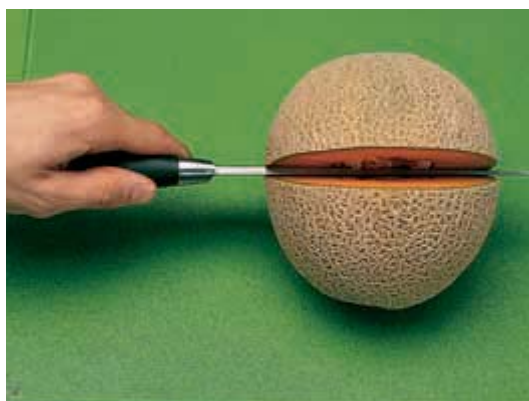
Figure 8 A knife is a common example of a wedge, a simple machine consisting of two inclined planes back to back.
